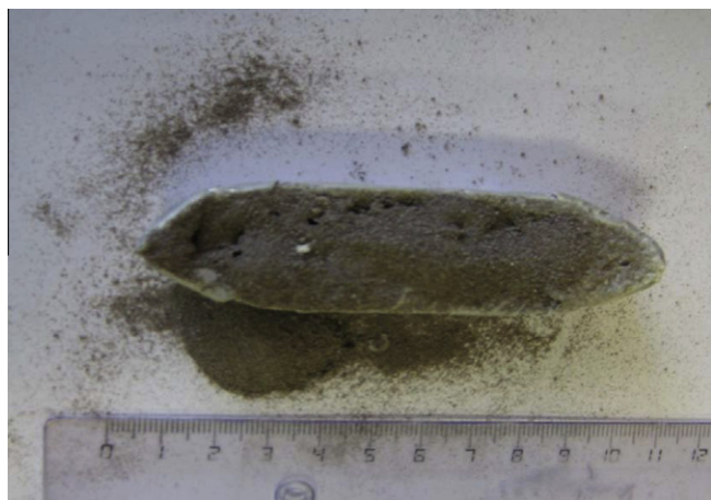
Fig. 3. Reaction container (made from Aluminium foil with dimensions length \sim 10 cm, width \sim 2.5 cm, height \sim 2.5 cm and thickness \sim 3 mm) containing sintered solid product of reaction of Finnish serpentine and AS.
