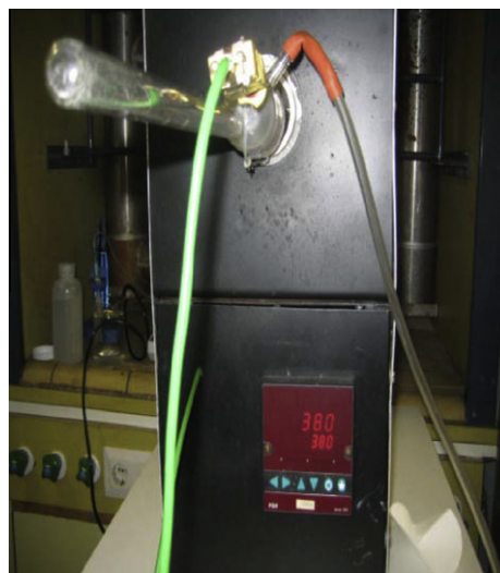
Fig. 4. Reactor/oven used for the reaction of serpentine and AS.
